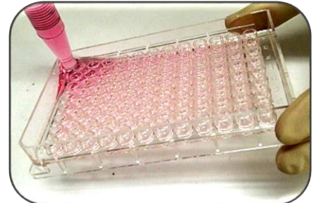
Easy one step media exchange by tilting the plate and aspirating from the corner.
